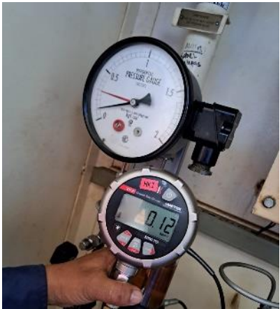
Gambar 8. Pengujian Differential Pressure Indicator
