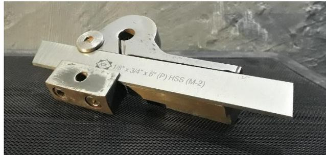
**Gambar 8.** Spring Parting Tool Holder
